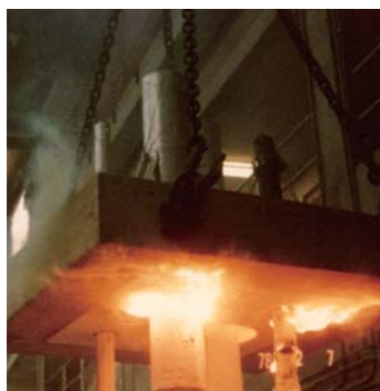
Test slab being raised from furnace at completion of test. (Slab was then positioned vertically for hose stream test.)
